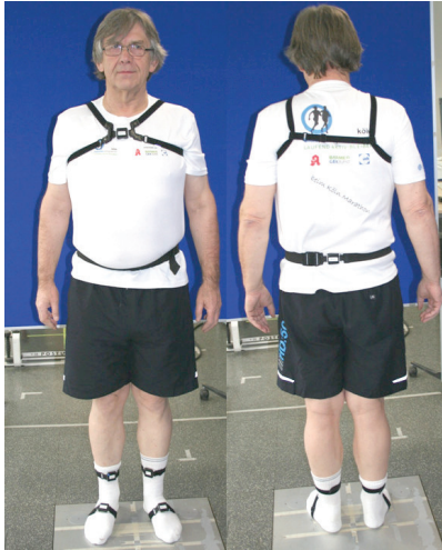
Figure 2. Movement sensor positions for balance ability measurement
