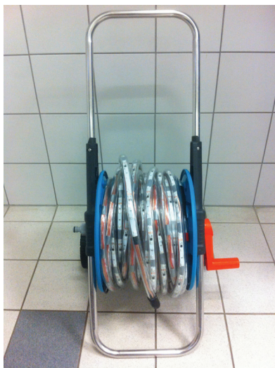
Figure 1. Swimming Pace Control System (SPCS) device before installation at the bottom of the swimming pool
