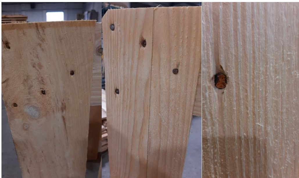
Figure 3. Fracture of structural elements of cargo pallets Source: own elaboration.
