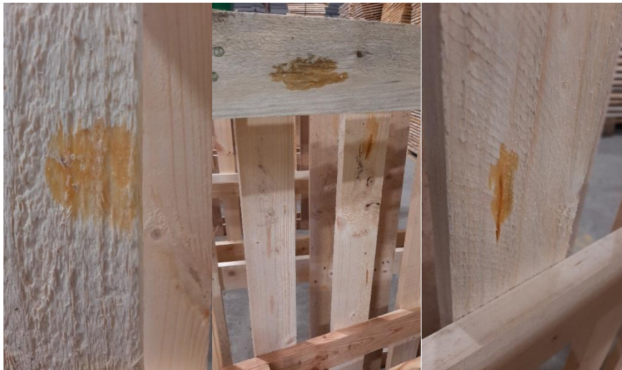
Figure 6. Resin leakage Source: own elaboration.
